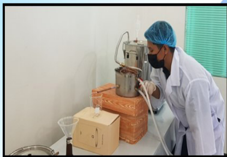
Distillation process and measuring alcohol content using alcometer
